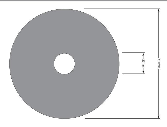
Printable area from 23mm to 118mm | This diagram is not to Scale
